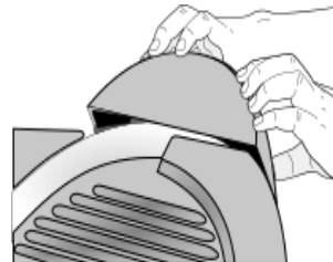
FIG 3. INSTALLING THE SHARPENER BOX
